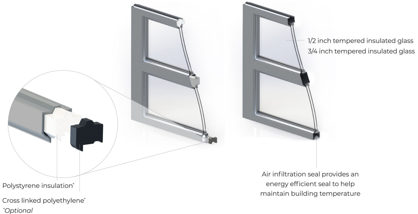
Insulated Stylist Cross Section*
